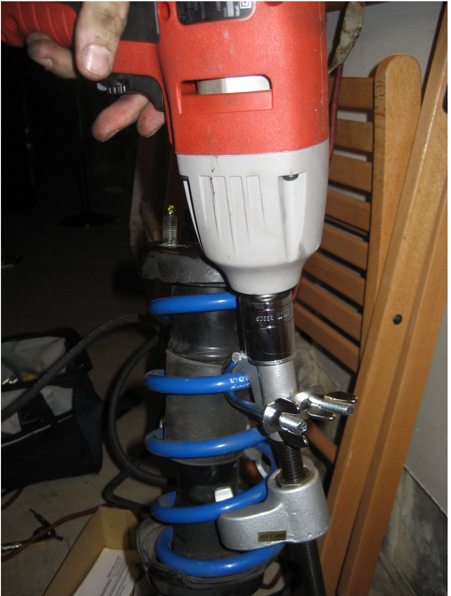
Once the compressors are on it should look something like this. Note the spring is compressed here - the bottom of the spring is no
