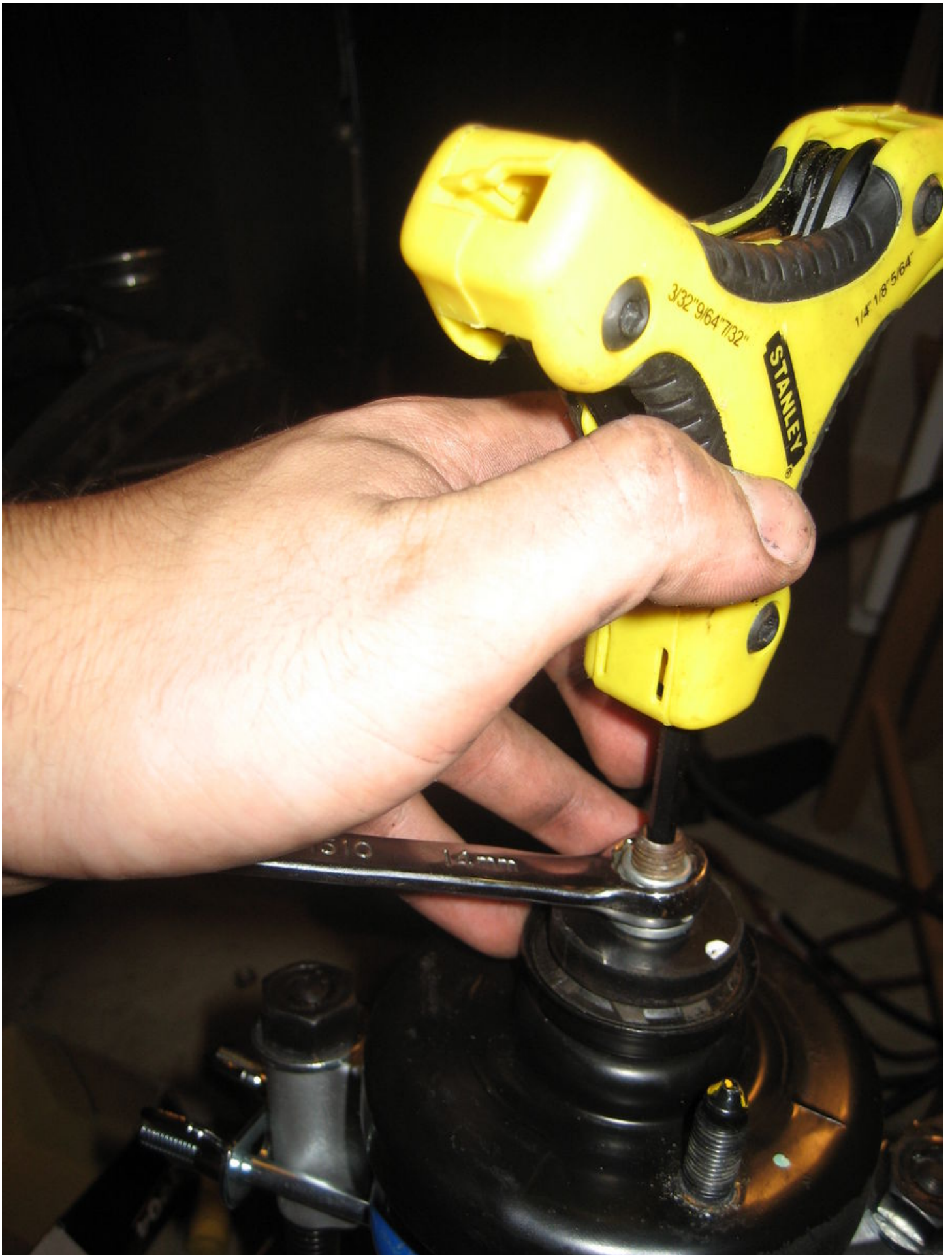
The next step is to put the top hat on to the new suspension. I did not pull apart the old top hat. I simply clipped it on to the KW
