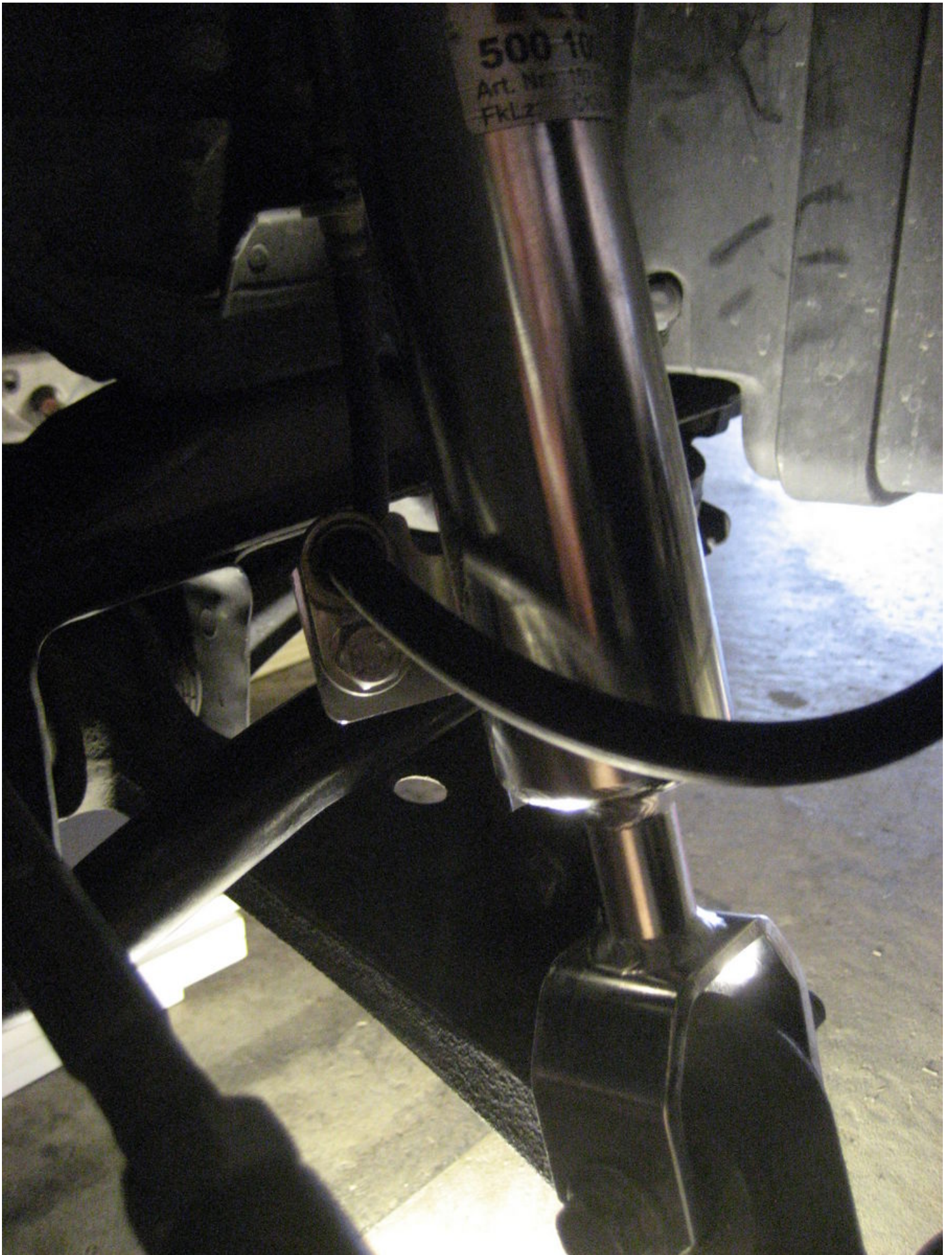
You are done with the drivers side - expect for torquing the top bolts - which we will do once the car is under load
